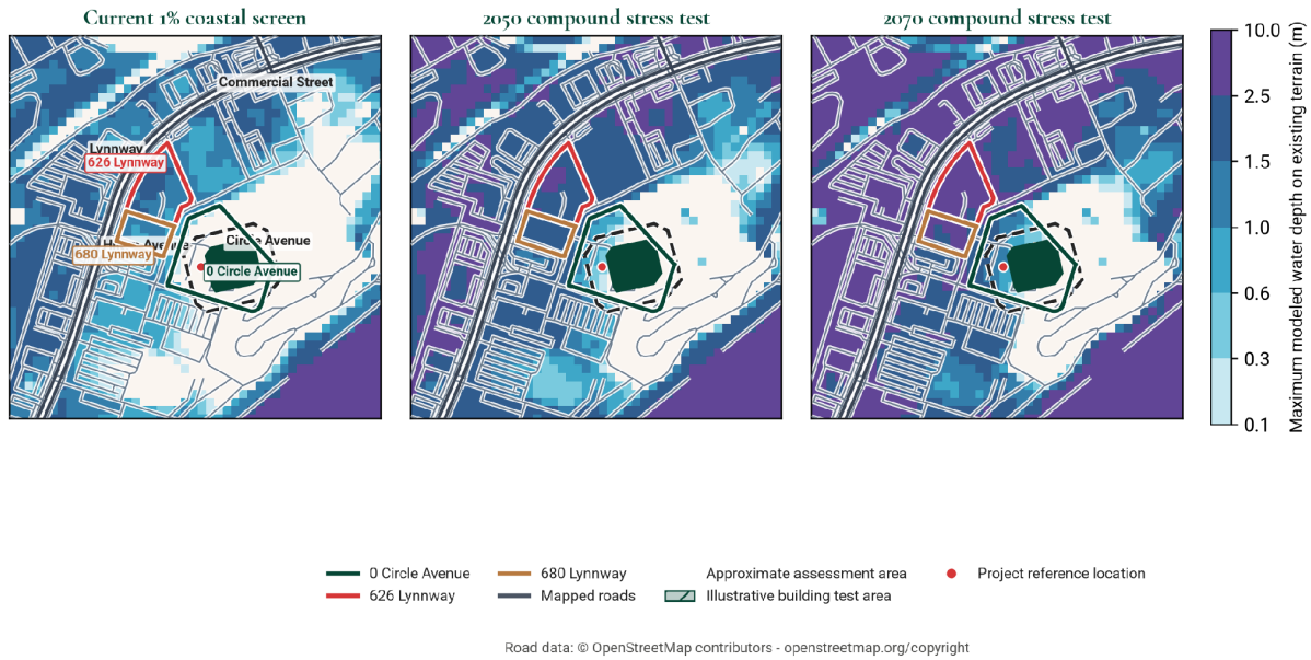
Figure 5. Arkadah flood-depth assessment with the three MassGIS parcel screening boundaries. Road source: © OpenStreetMap contributors. The 2050 and 2070 panels are compound stress tests.
